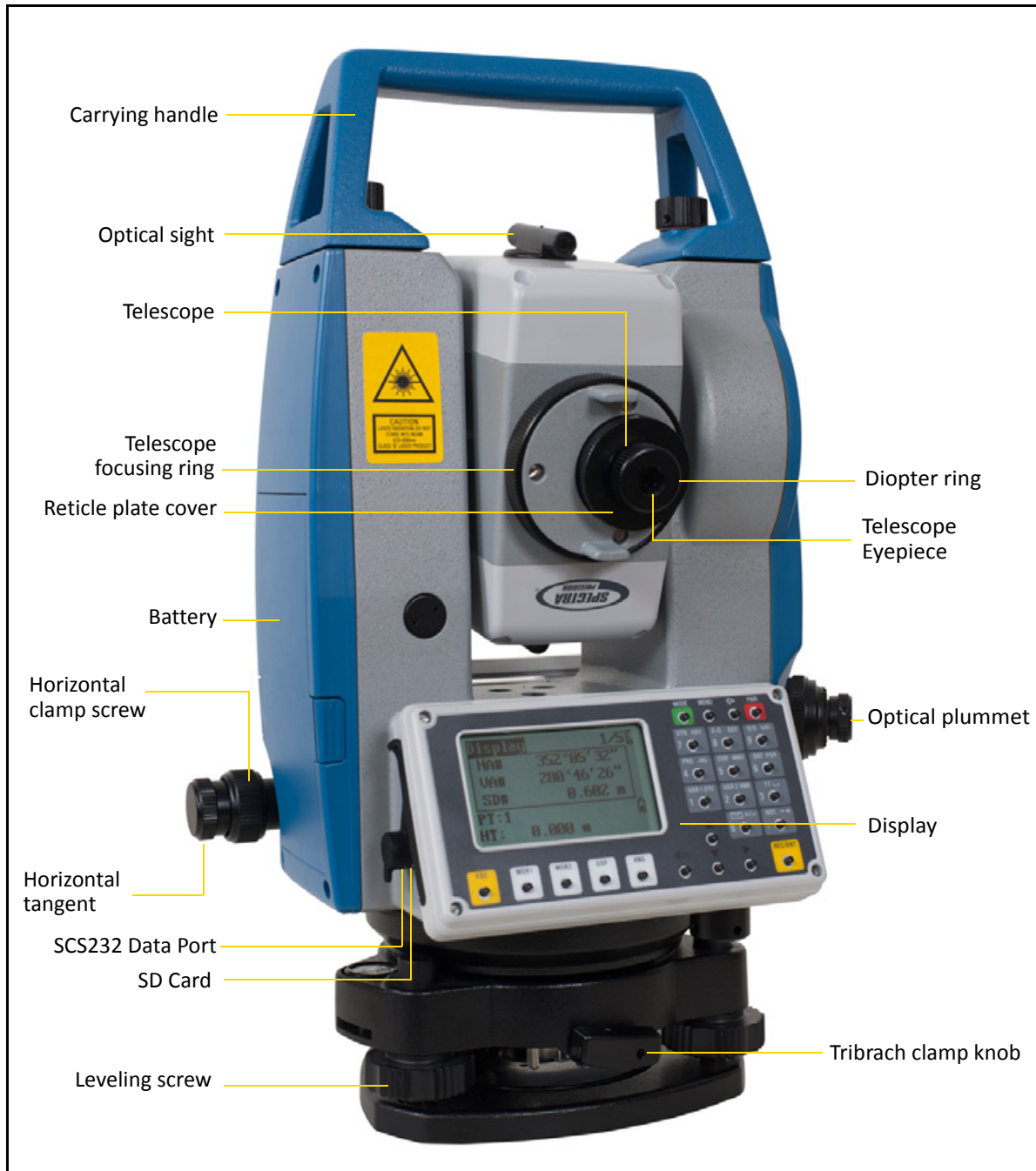
Figure 1.1 FOCUS 2 Series total station: Face 1
