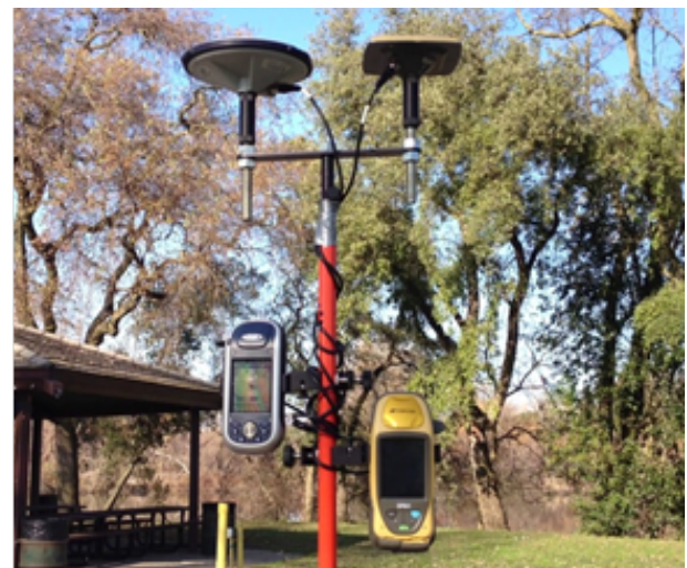
Figure 5: ProMark 220 and the competitive product fixed on the same rod, each using its own brand antenna.
