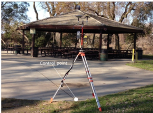
Figure 3: Test set-up over the control point (Point A).
